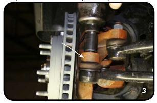
6. Remove the drag link at the knuckle using a 21mm socket and Hit the face of the knuckle with a ball peen hammer. (Photo #4)
