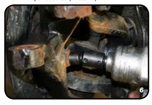
Remove the wheel speed sensor using a 5mm allen. (Photo #7)
