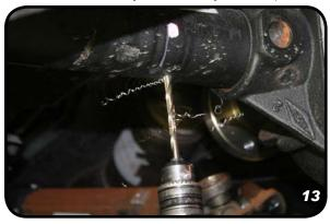
After pilot holes are drilled, drill holes out to ½" diameter so you will get good penetration on your plug welds. (Photo #14)
