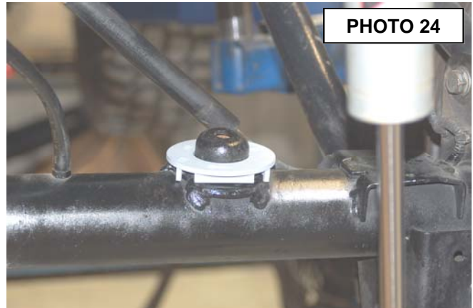
Install the lower control arms
