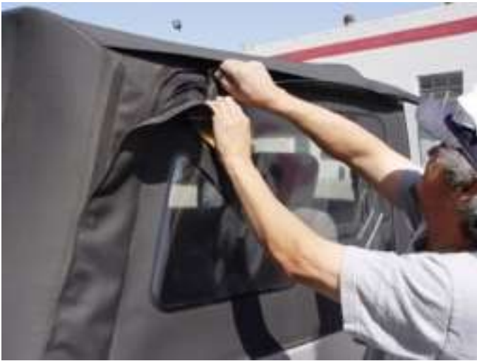
1. Remove side windows. (Left & right)
