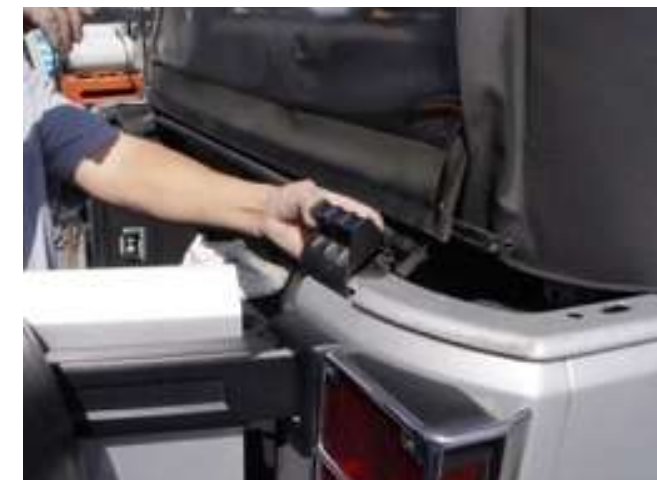
5. Remove retainers. (Left & right)
