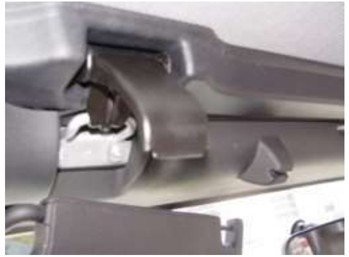
2. Disengage front clips and remove 2 screws holding the retainer loop. Remove loop. Both sides.
