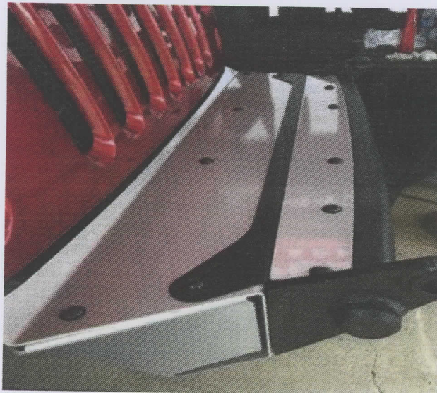
Figure 13: The front tube weldment attached to the main portion of the bumper
