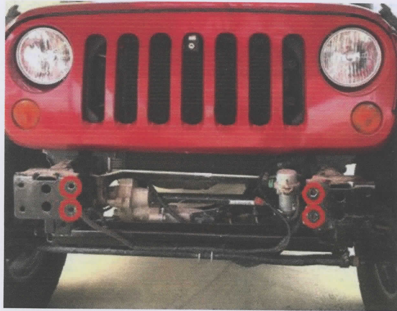
Figure 10: Red circles indicate where to install clip nuts
