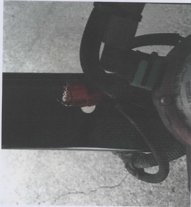
Figure 5: Wire loom and plug for the fog lights
