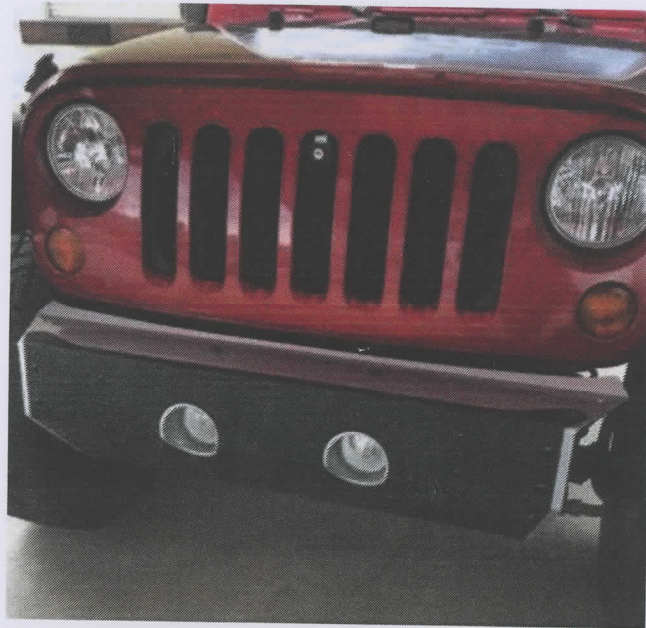
Figure 12: The main portion of the bumper resting on the stock vehicle mounts
