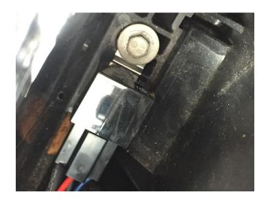
6. Install Power Supply and find a safe ground.
