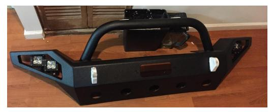
3. Lift Barricade Trail Force HD Full Width Bumper w/LED onto your vehicle. It's best to seek the help of somebody else when lifting and positioning the bumper. Place the OEM spacers you saved earlier on the back sides of the bolts and place the single, opposing bolts, lock and flat washers onto the bumper.
