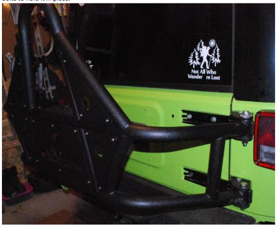
15. Swing the carrier open and install the tire stud and license plate holder with the six (6) 12mm bolts provided.
