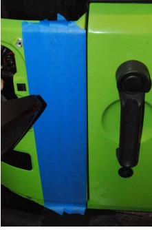
18. With the tire mounted to the carrier (to ensure proper weight), attach the tire carrier body bracket to the doorside of the new carrier by inserting the two (2) quick release pins (with the rectangular handles). Gently close the new carrier so that the body bracket lines up properly to the body, and use a pen or marker to mark where the five (5) holes are in the bracket. Mark precisely, because this is where you will drill into the body.
