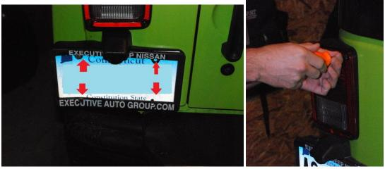
13. Disconnect the wiring from your license plate holder to remove. Tuck the wires into the body of the Jeep. Install the license plate holder delete plate using two strips of 3M double-sided adhesive tape (included).
