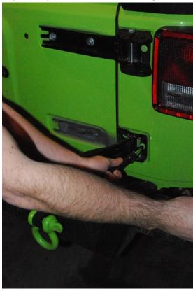
11. Place the hinge stopper bolt into the top hinge. (keeps carrier from swinging out too far) Hinge Pin Hinge Stopper Bolt Under side 12. Using a 9/32" nut driver, remove the four (4) license plate bolts. Remove the four (4) bolts from the tail light above the license plate as well.
