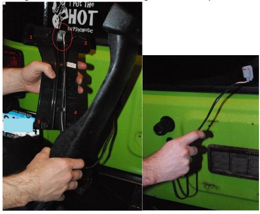
b. If you do not wish to use the original brake light wiring in the future, open the tailgate, pop out the plastic cover (shown below) and unplug the grey wire connector.
