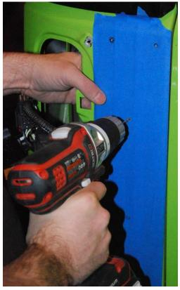
20. Remove the painters tape and close the tire carrier. Use the provided hardware to mount the bracket to the body with 5/16" bolts, and secure with nuts on the inside of the vehicle body.
