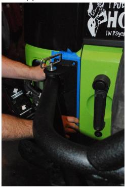
19. Gently use a center punch and hammer to mark the center of your mounting marks. Using a 1/8" drill bit, drill pilot holes into the five (5) marks you have made. Once the 1/8" pilot holes are drilled, use a 5/16" drill bit to drill out the five (5) holes. (Note: In some areas, you will be drilling through two layers of sheet metal)
