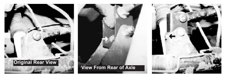
14. Check Brake Line Length, if they seem too short, longer stainless steel DOT Approved lines are available from Skyjacker. A driveline vibration may occur. If so, a transfer case lowering kit from Skyjacker should be installed.
