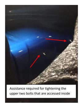
5. Continue fastening the remaining three bolts using the 8mm socket and allen wrench.
