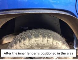
3. Using a center punch or a marker, mark the holes in the fender to be drilled. Either remove the fender or carefully drill through the holes in the inner finder assembly. Note: on drivers side take extra care to not drill through fuel lines. Note: jack may be used to provide better access for drill.
