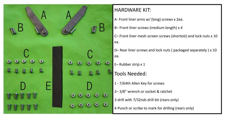
\*Special Note: You will need to save and re-use the 8 factory 10mm bolts that held the factory liners in the front.
