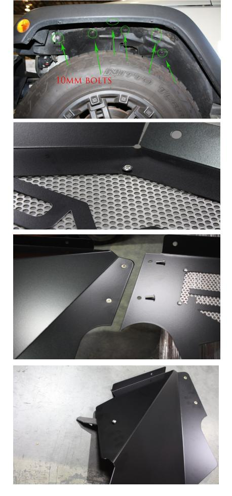
5) Place the liners in the fender location. You will use the factory hardware to attach to the Jeep at the four locations indicated by arrows. Cut and use the supplied adhesive rubber strip (E) to dampen any noise made from metal on metal contact if needed.
