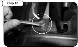
Secure core support bracket using 13mm.
