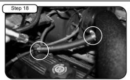
Reinstall crankcase line using the supplied 5/8" hose and mini clamps and attach to engine and intake tube. Secure mini clamps using 1/4" nut driver.
