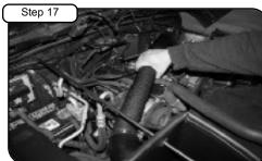
Attach straight coupling with #044 clamps provided on end of intake tube and position to housing and throttle body.
