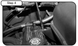
Loosen bolts holding in stock intake tube on valve cover using 8mm socket or wrench and remove.
