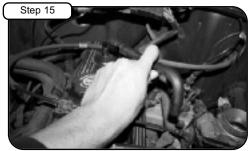
Remove crank case line from engine.
