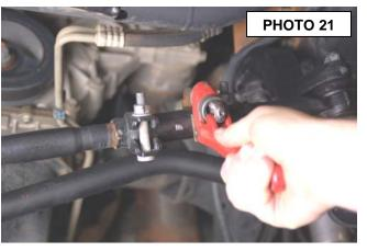
IMPORTANT NOTE: The draglink must be adjusted to the center steering wheel <u>BEFORE</u> the vehicle is driven. Failure to do so will cause a computer error, odd handling, and poor performance.
