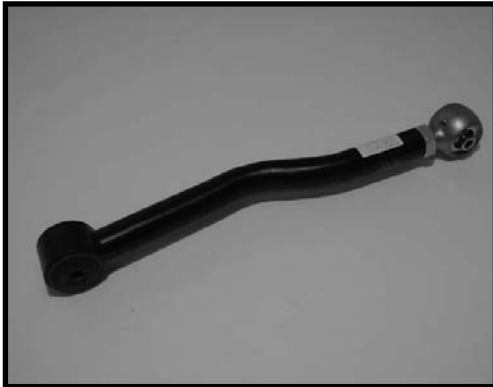
44000-01 (1) DS EZ-Flex front lower control arm
