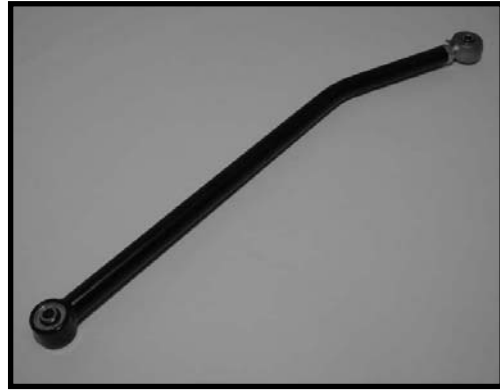
44000-07 (1) Front adjustable track bar
