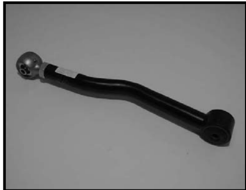
44000-02 (1) PS EZ-Flex front lower control arm
