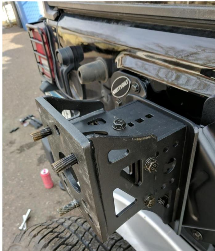
6. Re-install the spare tire and hook up the third brake light.
