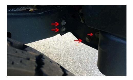
7. After you loosen all bolts, remove the zip tie holding the trailer wiring harness to the bumper before removal.
