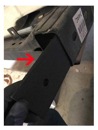
Make sure the side of the nut plate that has the nuts on it is flush with the outside of the frame.
