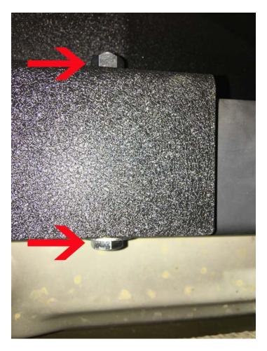
You will want to thread the bolts from the front of the Jeep to the back of the bumper. Get all the bolts threaded through and then add all the nuts, washers and spring washers.
