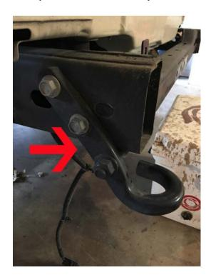
This step requires you to remove the two side bolts and a bolt underneath the tow hook.
