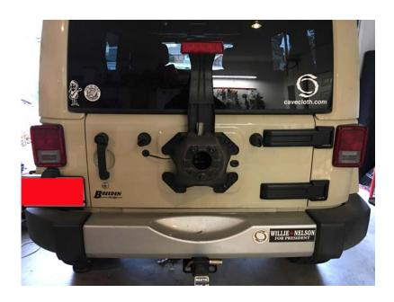
6. Remove the original bumper by unbolting the two bolts on either side of the bumper just inside the wheel well to the back using a 19mm socket.
