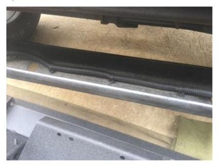
11. The bumper can then be placed onto the chassis. Put the washer onto the screw, that is attached to the bumper, then put the lock washer on, and finally the 18mm nut.
