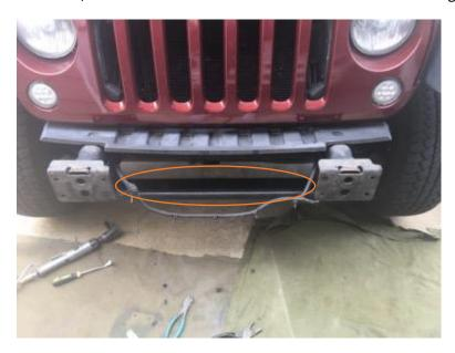
10. I drilled holes into this metal are to stick the clips into. NOTE: You do not need to drill these holes. You can tape them into this area, which would be sufficient.
