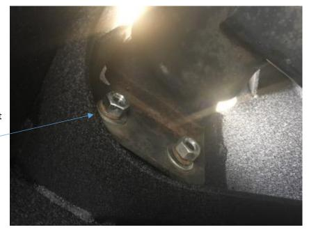
Here is the correct setup of the washer, lock washer, and nut
