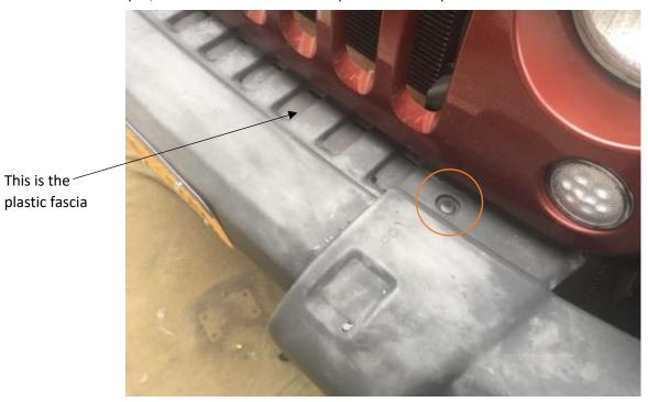
6. Begin to remove the eight factory nuts from the front bumper using the 18mm socket and socket wrench.
