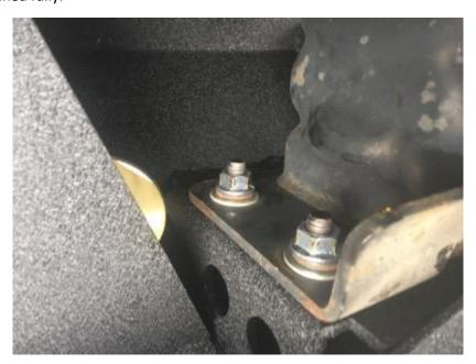
13. This is what the fully installed bumper will look like before the D-Rings are put on. NOTE: I have placed a license plate carrier on the bumper already, this will not be included with the bumper.
