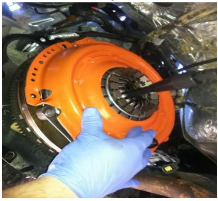
27. Install New Centerforce Pressure Plate by tightening 6 bolts included in kit to the specified torque setting stated in the kit. NOT OEM TORQUE LEVEL.
