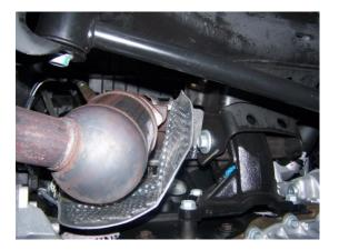
2. NOW STARTING UP TOP ON THE DRIVER SIDE, REMOVE STEERING SHAFT FOR REMOVAL OF FACTORY MANIFOLDS AND INSTALLATION OF HEADER. DISCONNECT ALL SPARK PLUG WIRES, REMOVE FACTORY HEAT SHIELDS AND MANIFOLD. MAKE SURE CYLINDER HEAD SURFACE IS CLEAN OF ANY DEBRIS BEFORE INSTALLATION OF HEADER.
