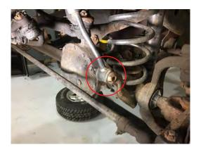
Place the floor jack under the front axle to provide support. Remove the factory shock. Retain the factory mounting hardware ((2) 13mm bolts) these will be reused with the Mammoth shock.
