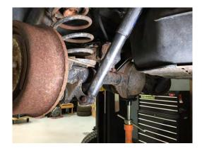
Place the floor jack under the axle to provide support. Remove the factory shock. Factory hardware as it will be reused.
