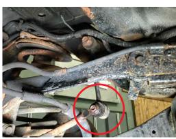
Slowly lower the rear axle to remove the factory springs. \*\*Note: The differential vent tube may need to be unclipped to prevent strain when lowering the axle. A spring compressor may be needed to remove the factory spring.
