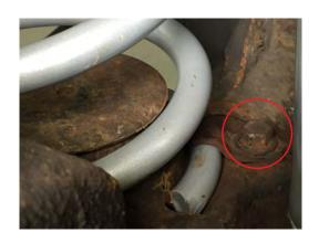
Install the supplied shock using the factory lower bolts. Use the supplied washers and bushings on the upper mount.
