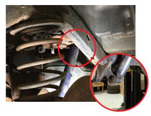
Remove the end link from the sway bar.
