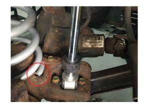
Re-install the factory spring clamp.
