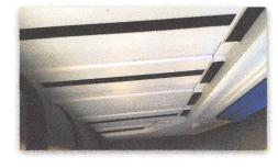
adhesive time to set up. Then once again reapply pressure to the velcro strips! Position headliner and press them into place. Extra Velcro is included if you need it.
