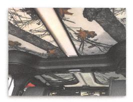
Step 1: After unpacking and before removing the protective white backing on the Velcro test position each panel. The rear seat Headliner panel will slide up and tuck over the speaker bar just slightly. This is intentional to assure good insulation and a tight fit!
