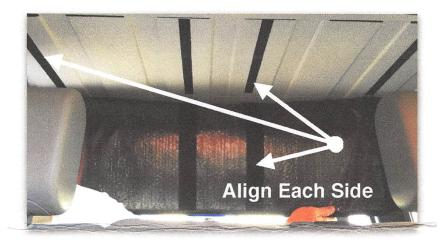
**Step 3:** Check the Velcro alignment, **remove** the velcro strips from Headliner and press them firmly
