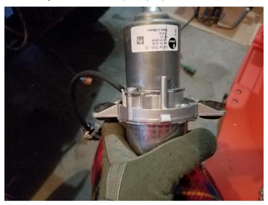
**15.** Using the supplied hardware, 10mm socket, and 10mm wrench, attach the vacuum pump to the underside of the winch plate as shown. I recommend adding a large washer so the nut doesn't sink into the bushing.
