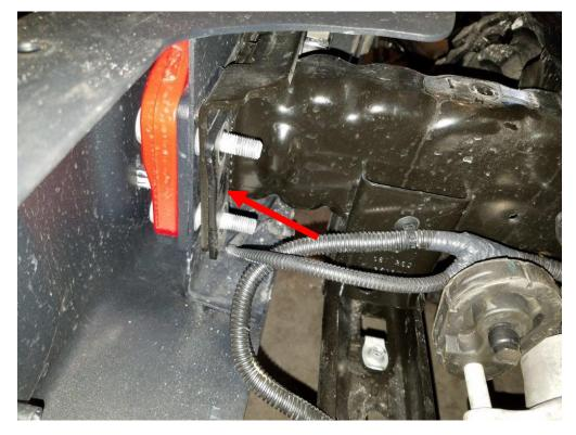
**7.** At this point you should have removed 8 nuts, and 4 backer plates that hold on the bumper. Now you can remove the bumper. Lift the bumper by holding the stock tow hooks. Make sure you have a soft place to put the bumper so it doesn't get damaged.
