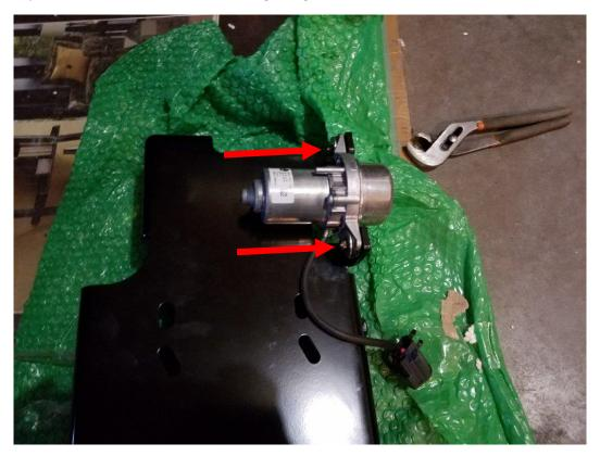
**16.** Insert the winch plate between the frame horns as shown below. Then reconnect the 2 hoses and wire harness removed from the vacuum pump. *Note: You can see below there are 2 sets of winch mount holes. The straight holes are for offset mount, and the diagonal holes are for centered mount. You will need to choose the holes that work for your specific setup.*
