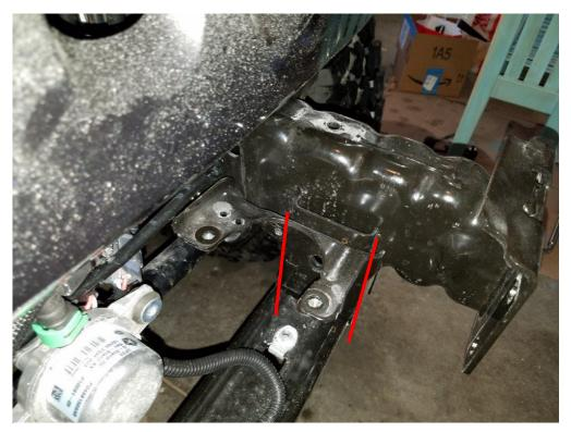
**12.** Once you have removed the bracket it should look about like this. I recommend using the grinder to smooth out the sharp metal edges. Then use black spray paint to cover the bare metal. This will help prevent rust.
