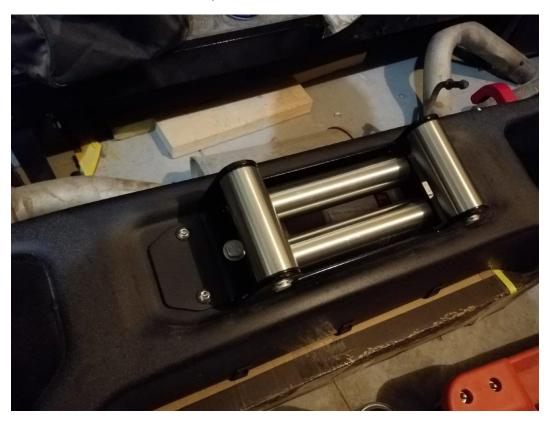
**21.** Disengage the winch clutch and pull out a foot or so of cable, then reengage the clutch. With the weight of the winch these 4 bolt holes may not line up perfect. Be prepared to lift up on the winch as you are installing the bumper.
