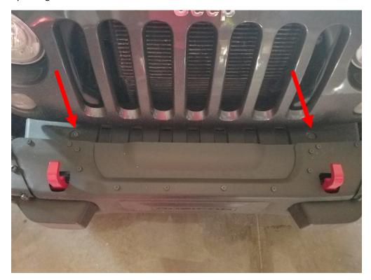
2. Next, using a wrench with a T30 star bit, remove the 8 bolts holding the winch cover plate. Then remove the plate.
