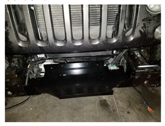
**17.** Insert the upper winch bracket as shown below. Install the 4 supplied bolts and washers. Just hand tighten for now.
