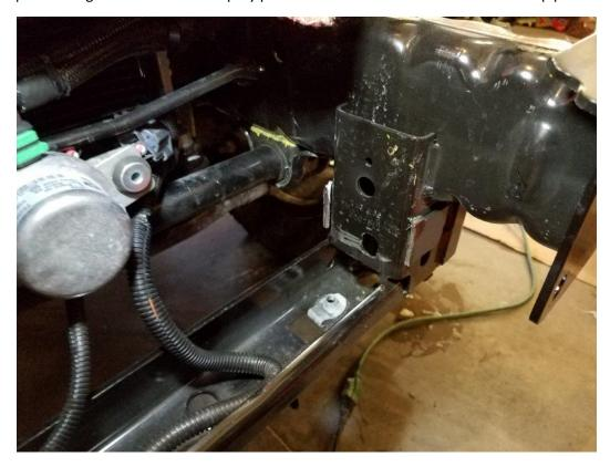
**13.** I found that the supplied bolts are not long enough to hold the pump if you use the stock bushings. I recommend you remove the metal sleeve from inside this bushing, then use a utility knife to trim about ½" off the thick side of the bushing.
