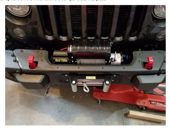
**23.** Install the winch hook with the supplied cotter pin to keep the cable from pulling back through.
