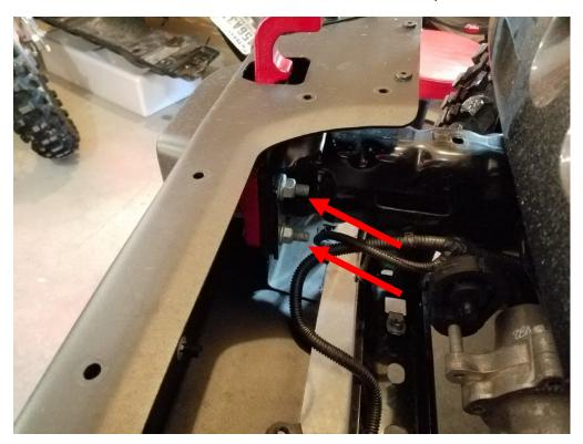
**6.** Then remove the backer plates under the nuts.
