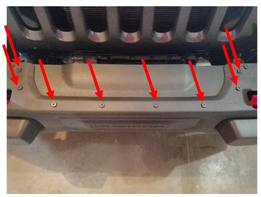
**3.** Using a 16mm socket, remove the 7 bolts holding on the front skid plate, and remove the skid plate.
