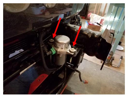
**10.** Disconnect the wire harness, the drain tube, and the vacuum tube. The vacuum tube can be removed by lifting the 4 tabs on the green connector shown below. Then place the vacuum pump aside.
