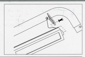
2. Attach LH and RH brackets to crossbar with supplied M10 button head bolts, M10 Flat Washers, and M10 lock nut. Do not tighten completely to allow for adjustment.
