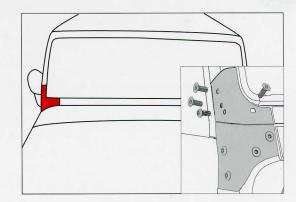
4. Install assembly to vehicle using supplied 5/16" button head bolts and washers. Adjust fitment if necessary and securely tighten all bolts.
