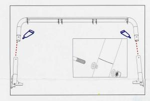
3. Using a T40 Torx driver, remove the 4 factory bolts from the upper portion of the LH and RH windshield hinge.
