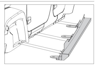
**NOTICE** Have someone help lift the Rock Slider into place to avoid damaging the vehicle.
