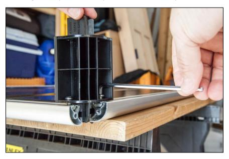
14. Insert one #332 bolt into each of the pre-drilled upper holes of the composite corners. Apply thread locking compound and loosely attach one #651390 T-Nut to each of the bolts with the beveled side of the T-Nuts facing up. Orient the remaining short and long rails with one channel facing the interior of the cargo rack and the other channel facing down. Slide each rail into place by inserting the T-Nuts into the bottom channel.
