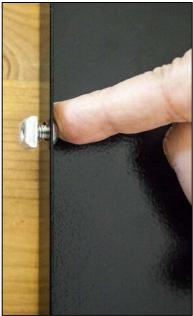
6. Flip the panels over. Orient one of the shorter #820004 rails with one channel facing the beveled T-Nuts and the other channel facing up. Attach the rail by sliding each of the T-Nuts into the side channel of the rail. If the rail binds, loosen the T-nuts and/or reach under the panels to hold the bolt heads against the panel edge to create a larger gap for the rail.
