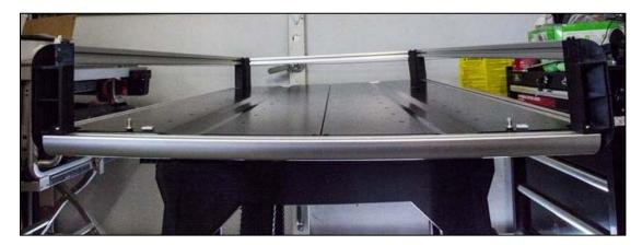
15. Flip the cargo rack upside down so the just installed rails are resting on the large flat surface. Square up corners and tighten all eight bolts. Torque each one to 5 ft-lbs.
