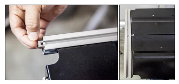
8. Insert one #332 bolt into each of the two lower, pre-drilled holes of the #820002 composite corners. Apply thread locking compound and loosely attach one #651390 T-Nut to each of the bolts with the beveled side of the T-Nuts facing away from the composite corner body.
