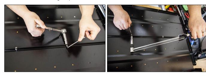
5. Insert 18 #333 bolts through each of the pre-drilled holes along the perimeter of the conjoined panels. The bolt heads should be facing the center of the panels. Apply thread locking compound and loosely attach one #651390 T-Nut to each of the bolts with the beveled side of the T-Nut facing out.
