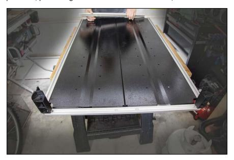
12. Attach the remaining two #820002 composite corners by inserting a #651390 T-Nut into each end of the exposed upper channel rails (total of four).
