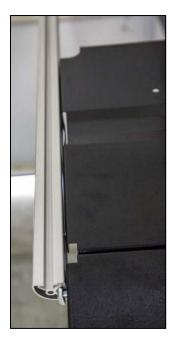
7. Once the rail is attached, slide two T-Nuts into the top channel, positioning them near the middle of the rail, for future use.
