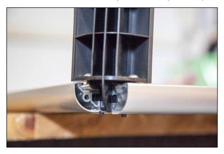
11. Orient the second short #820004 rail with one channel facing the beveled T-Nuts and the other channel facing up. Slide the rail into place by inserting the T-Nuts into the side channel. Once the rail is attached, slide two T-Nuts into the top channel, positioning them near the middle of the rail, for future use.
