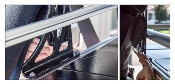
22. Position the rack front to back to desired location within cargo area, ensuring there is at least a ¼" gap between the rack and the back of the rear Jeep seats. Using the allen wrench, tighten the cargo rack bracket bolts. Torque each to 5 ft-lbs.
