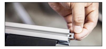
13. Insert one #332 bolt into each of the two lower, pre-drilled holes of the #820002 composite corners. Apply thread locking compound. Adjust rails and corners to ensure they are square and evenly spaced. Using the supplied allen wrench, tighten all panel and composite corner bolts. Torque to 5 ft-lbs.
