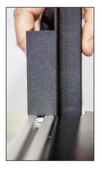
10. Orient one of the longer #820003 rails with one channel facing the beveled T-Nuts and the other channel facing up. Attach the rail by sliding each of the T-Nuts into the side channel of the rail. If the rail binds, loosen the T-nuts and/or reach under the panels to hold the bolt heads against the panel edge to create a larger gap for the rail. Slide the rail onto the second T-Nut from the composite corner. Repeat install process for second long rail.
