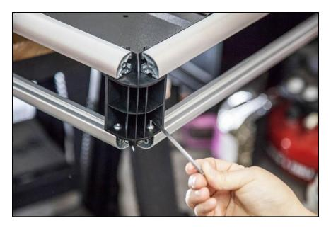
16. Attach the 4 #820001 composite corner covers by aligning two clips on one side and then rolling the cap toward the other set of clips until the cover snaps into place. If you're having difficulty attaching the covers, verify the cargo rack rails are square and try again.
