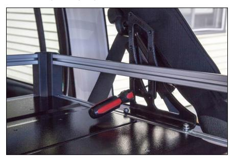
21. Apply thread locking compound to three #330 bolts and insert them through the pre-drilled, pre-threaded mounting holes of the roll cage bracket on the driver and passenger sides. Ensure the rack is level. Using the allen wrench, tighten all of the bolts. Torque each to 5 ft-lbs.
