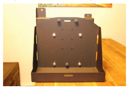
Be sure to mount the tray with the nuts on the back side of the mount to ensure the bolts will not contact and damage the container placed in the tray.
