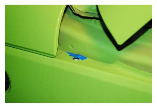
5. Remove the lower bolt from the windshield bracket using the T45 Torx Driver. Please note that the windshield bracket on the jeep in the pictures is black power-coated because it is part of a previously installed light bar. The stock windshield bracket will be body-colored.
