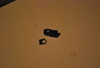
4. Using the Needle Nose Pliers, carefully hang the J-Nut from the fender making sure the threaded nut is visible through the square hole in the fender. You can help secure it from slipping off with a small piece of masking tape.
