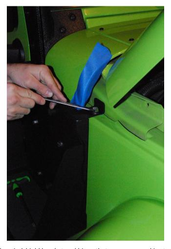
8. Reinstall the bolt into the windshield bracket and hinge that were removed in steps 5 and 6 through the mount.
