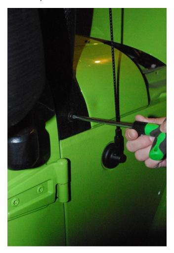
6. Open the door and remove the top bolt from the inner hinge using the 13mm socket and ratchet.
