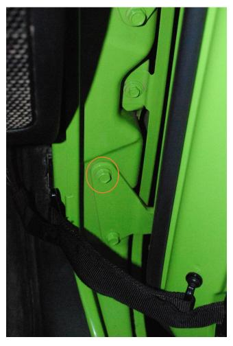
7. With the help of a friend, hold the mount in place over the three holes. Install the included bolt and washer through the top hole of the mount and into the J-Nut. Leave the bolt loose. Note that some masking tape was put on the front of the cowl to protect the paint. This is not strictly necessary, but the fit is tight and it is recommended.
