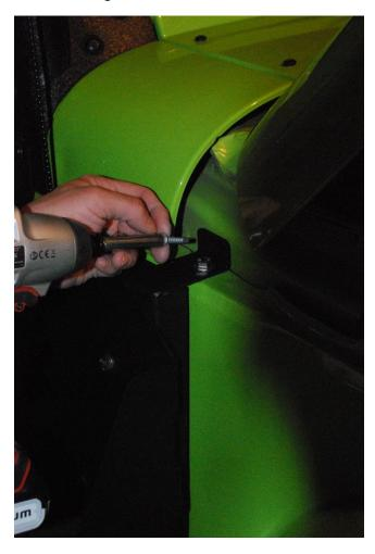
Post Installation: Verify the mount is secure. Close the hood and door carefully and check for clearance. Using the provided strap, install the desired container and verify clearance with the door and mirror. Enjoy your MORyde Side Mount Tray!
