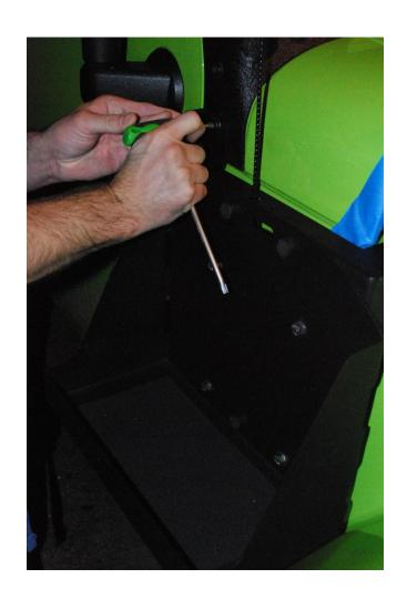
9. OPTIONAL: For additional strength, a self-tapping screw is included that can be used to attach the tab at the top of the mount. This can be installed using a drill or electric screwdriver.
