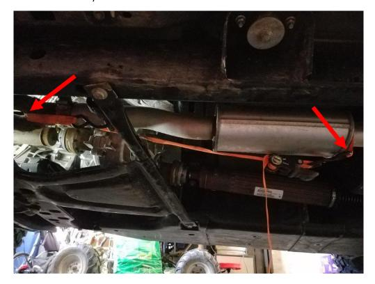
**6.** Using a 13mm socket remove the 4 bolts holding the 2 exhaust joints together. You may need penetrating oil on these bolts to loosen them if your exhaust is older.
