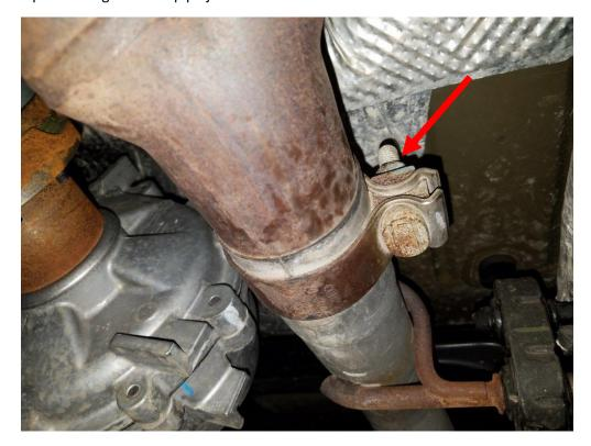
2. Next you will need to remove the small metal index tab shown below. Steps 3-4 will detail how to remove it.
