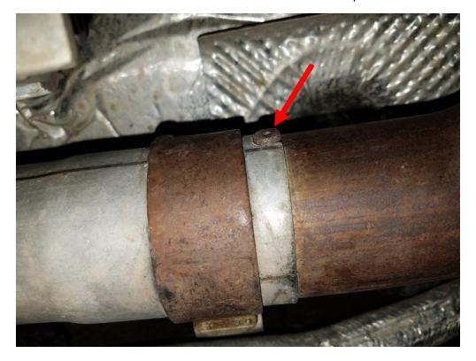
**3.** Attach a ratchet strap from the exhaust hanger to the frame as shown below. Then tighten the strap until the exhaust joint shown pulls apart a few inches. This will give you the room to remove the index tab. Note: If you have trouble with this step, make sure to use extra penetrating oil in the exhaust joint and give it time to soak in.
