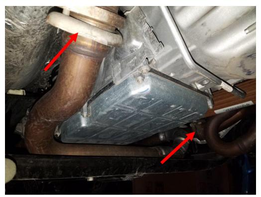
7. The top bolt on the left hand joint is hard to get to, I recommend using a long socket extension as shown below.
