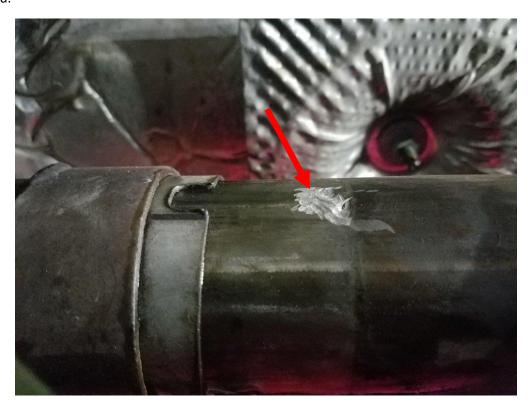
5. Next, attach a ratchet strap from the Y-pipe to the resonator as shown below. Tighten the strap until the mid pipe slides back over the Y-pipe. You want it to slide past the point where it covers the spot of the removed index tab. This is the reason you removed the index tab.
