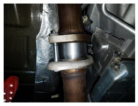
**10.** Last, using a 15mm socket, retighten the midpipe connector and any other exhaust parts you loosened. *Note: I recommend you check and retighten all hardware after driving a few hundred miles.*
