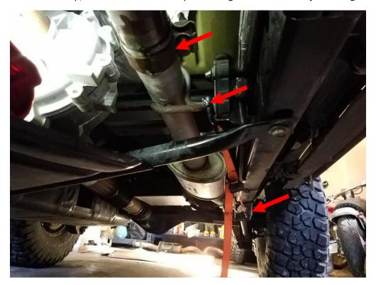
**4.** Next use a dremmel with a metal cutoff wheel, or a sawzall to remove the small index tab from the Y pipe. Take your time and grind it smooth, it is a tight spot and hard to work in. It should look something like this once it is removed.
