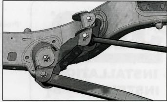
**Note:** It may be easier to align the control arms to the mount by removing the opposite side upper control arm and adjusting the axle with a hydraulic jack.
