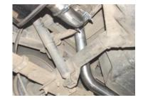
Next install over axle tailpipe #C onto pipe #B. Install hanger # F and slide hanger into rubber grommet. Use clamp #E to secure pipes together. Do not tighten. After checking for your proper clearness tighten all clamps starting from the front and working your way to the back.
