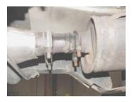
Lay out the exhaust on the floor so it looks like the drawing and compare parts with manual. Remove the stock exhaust from the clamp located between the catalitic converter and your muffler. You may need to heat it up for easier removal. Leave all rubber grommets in place. Use WD-40 to aid in removal of exhaust and hangers. Use hacksaw to cut muffler and tailpipe off.
