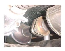
LAY OUT THE GIBSON EXHAUST ON THE FLOOR SO IT LOOKS LIKE THE DRAWING AND COMPARE IT TO THE MANUAL. TO REMOVE THE STOCK EXHAUST CUT OFF TAILPIPE JUST BEHIND THE MUFFLER. REMOVE THE MUFFLER FROM THE 2- BOLT FLANGE JUST IN FRONT OF THE MUFFLER, LEAVE ALL RUBBER GROMMETS IN PLACE, USE WD-40 TO AID IN REMOVAL OF EXHAUST AND HANGERS.
