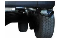
4. Install Metal Mulisha tips. Clamp down. When you have everything in place, firmly tighten all bolts and clamps down securely. Inspect all fasteners after 25-50 miles of operation and re-tighten as necessary.
