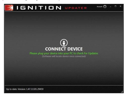
4. Connect the Flashcal device to your computer using the provided USB cable. The screen of the Flashcal device will display "USB Mode" when properly connected to the computer and the software will automatically attempt to locate and install drivers for the Flashcal device.
