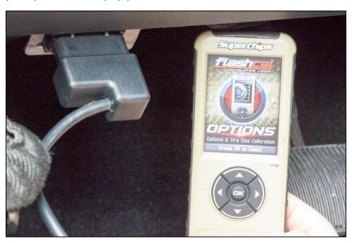
13. Insert the Jeep key into the ignition, but do not start the Jeep. Turn the key clockwise to the "On" position based on findings from Step 8.
