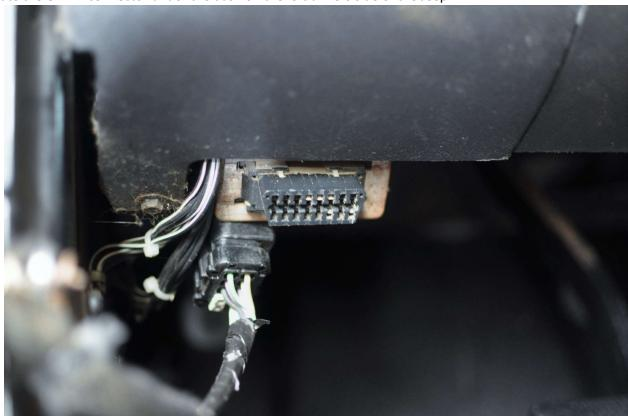
3. With the Jeep ignition key in the OFF position, connect the Flashcal to the OBD-II connector. Note: Do not remove or bump the OBD-II connector while changing settings on your Jeep. If you do, the Jeep may not start.
