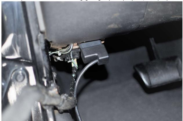
4. The Flashcal will power up and prompt you to turn the ignition key to the ON position (key position just before starter engage position). Press the OK button on the Flashcal once the ignition key is in the ON position.
