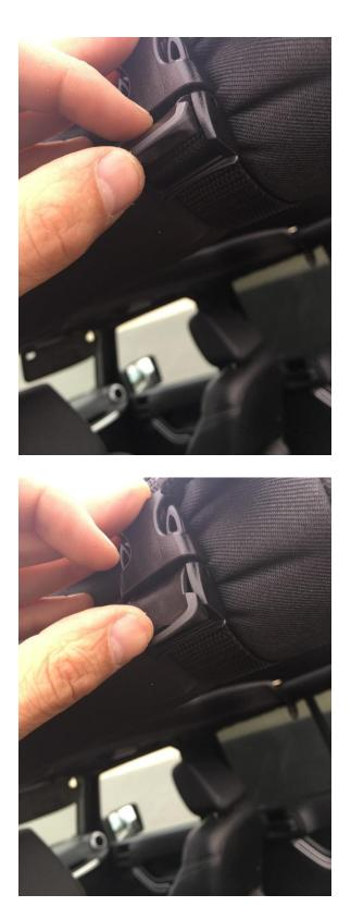
4. Once you have all the straps attached, starting again from the front, and working to the rear of the vehicle, tighten each of them, and secure the clip. Once I had done this, I took the excess strap and tucked it under the roll bar, so that it was not dangling.
