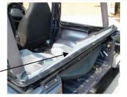
Lay the top fabric, backing side up in the rear of the vehicle with the plastic strip facing up and aligned with the front edge of the header. Locate the round hole that marks the center of the plastic strip (all other holes are slotted). Install a screw in the round hole to secure the fabric to the header as well as to center the top. Then proceed to install screws in the remaining seven or thirteen holes along the front of the header.
