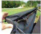
Step (4): Raise the header and bow assembly towards the windshield and into position. Inside the top, snap the fabric to the rear bow (total of six snaps).
