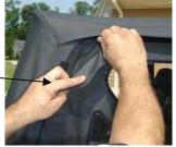
Step (12): Remove the rear window from the box and lay it flat with the backing side up. Locate the tailgate bar set aside in step one. The bar has a "C" shaped channel, when viewed from the end. Orient the bar with the round seal down and slide the "C" channel on the retainer onto the tubed strip sewn to the backing side of the rear window.
