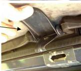
Step (7): Wrap and fasten the hook and loop on the two flaps inside the top around the center bow.
