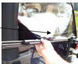
Step (2): Release the latch that secures the header to the windshield. Pull up on the lever and then down and out to release the hook from the slot in the windshield frame.
