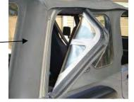
Step (2): Release the front of the top from the windshield. Raise the front of the deck and collapse the rear bows, tucking the two plastic strips above the door opening and the stay pad on the rear bow inside of the bows. Wrap the fabric around the bows, then tuck the rear legs of the top under the bows.
