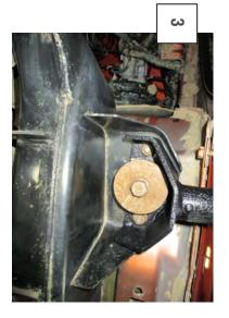
Slide the side step on top of the body mount and on to the threaded studs. Secure the side step using the factory hardware and torque to 40 filhs
