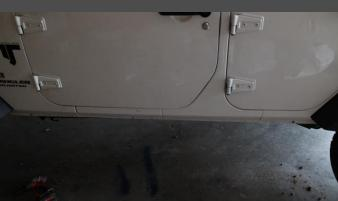
c. After Stock bolts are remove pull the stock rail directly away from the body being careful to not scratch or make contact with the body of the Jeep.
