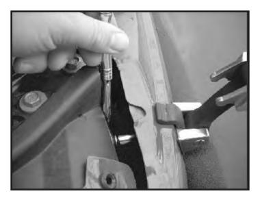
1. Remove the 13 mm retaining nut on the back side 2. Install the light mounting bracket with the mounting pointing towards the rear of the vehicle. Repeat this for both sides.
