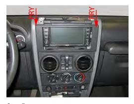
**Step 5:** Pry out on the top of the radio bezel. Pull the bezel away from the dashboard.
