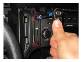
**Step 7:** Remove the (4) radio head unit retaining screws from the stock head unit. There will be (2) on each side of the head unit.
