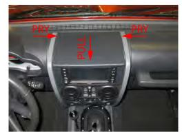
**Step 1:** Pry up both sides of the rear center dash cover. Once the back is loose, pill it toward you and remove from the vehicle.
