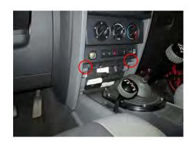
**Step 4:**Remove the (2) 7mm screws that are holding the bottom of the radio bezel.
