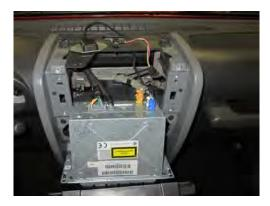
**Step 8:**The head unit can now be pulled from the dash, note the orientation of the wiring harnesses. The large plug is where the supplied jumper harness with be attached.
