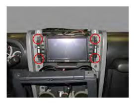
**Step 7:** Remove the (4) screws holding the head unit to the dash.
