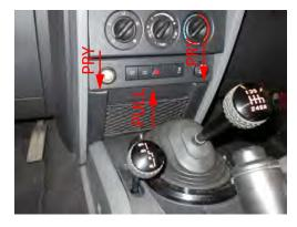
**Step 2:** Pry out the top of the netting trim. Once the top is loose pull up on the trim and remove it from the vehicle.
