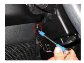
**Step 2:** Remove the (2) 7mm screws; there is (1) on each side of the steering column.
