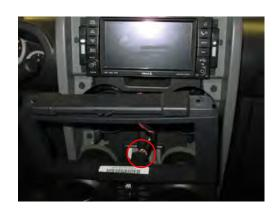
**Step 6:** Unplug the power window wiring harness if equipped.
