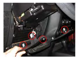
**Step 1:** Remove the knee bolster by pulling down on the top of the panel. The panel is hinged on the bottom and it will swing down, once the (4) metal clips release.
