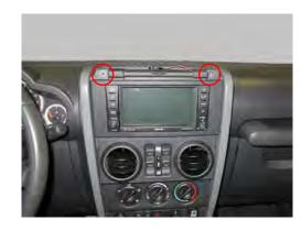
**Step 3:** Remove the (2) 7mm screws that are retaining the radio bezel.
