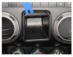
**Step 3:**Remove the center storage container/ window switches by prying the upper and lower tabs to release it from the radio bezel.
