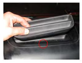
**Step 5:**Remove the upper dashboard storage tray by lifting it by the center tab. There is (1) 7mm screw underneath the removable
