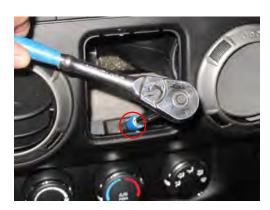
**Step 4:** There is (1) 7mm mounting screw at the bottom of the open area left from removing the storage container. Remove the screw.
