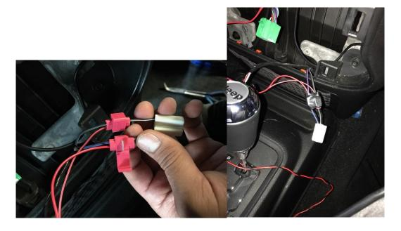
14. Next you will need to mount your LED. This LED will blink when you activate the NAV unlock so a passenger can enter an address while the vehicle is moving. Using the 5/16" drill bit select a location. I chose directly under the hazard button. It is out of the way but you can still see it flash off of the gear selector. The nut is a 10mm. I also cut the rubber covers in order to make it easier to slide the nut off of the LED.
