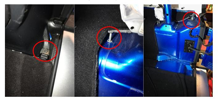
6. I chose to remove some of the zip tie/ Christmas tree fasteners that are used to keep the wires in place. If you cut them off and remove the loose piece and extra tab, you can feed your own ziptie through it and reinsert the Christmas tree fastener into the hole!
