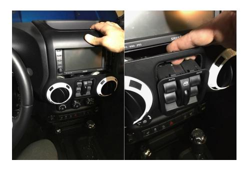
d. Turn the switch panel counterclockwise and unplug the harness by first sliding the red lock all the way to the left as pictured. Then depress the plug tab and remove the plug. Then remove the remaining 7mm bolt and remove the dash. (Tip: Lower your steering wheel as far as possible to help remove the dash)
