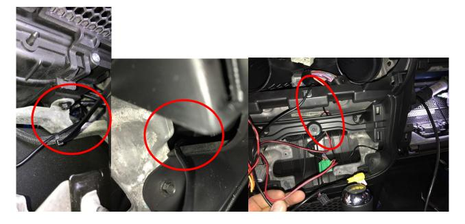
12. Now take the harnesses that came with the kit & attach them to the radio. BCI-CH21-AUX harness will have two yellow RCA Cables labeled "camera" plugged into eachother. Unplug them, your camera RCA will plug into the female that goes toward the radio. I decided to put the other harness into the dash before plugging it into the factory plug first due to its large size. Run the bulk of its cables around the radio frame and down the front toward the driver side temporarily.
