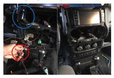
17. Replace your dash and all side panels. The last thing you will have to do is adjust the camera. I suggest pulling your jeep into a position with landmarks around (house or garage) for reference. Activate the "forced reverse camera" by holding the Preset button (center button on the back left of the steering wheel) with the jeep in park. Then with the rear glass open, I was able to see the screen and adjust the camera until it looked good.
