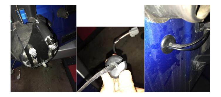
9. Zip tie the camera wires to your third brake light plug & run through the hole along the brake/lock lines. Take the RCA/ Power cable the kit came with and select the end with the yellow RCA & Black power plugs. (The side with the Yellow RCA & small Red and black wires will run to the front) I taped the RCA (yellow) & power (black) wires individually then together to hold them in place & Ziptied along the factory wiring.
