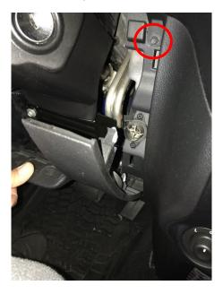
c. Gently pull back on center counsel above the stereo to pop the clips free. There is still one screw holding the bottom behind the window switches so carefully work the top free across the dash so you can see the back of the window switch panel. Once you can see the back of the window switches, reach behind it and push toward the inside of the vehicle to pop the panel out.
