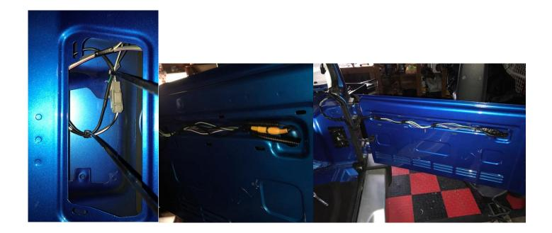
10. Follow the factory harness placing zipties every 6 – 12 inches. Keep the cable tight to factory harness (there isn't a lot of extra slack for the 4dr!) Once at the front passenger footwell, bring the cable up underneath the glovebox. Ziptie the cable to one of the ground wires there. Don't ziptie it to your door plug, or you will have issues next time you remove your doors! Remove glovebox by pressing on the sides.
