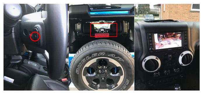
18. To activate the Navigation Unlock, Hold the Source button (behind the right side of the steering wheel). Your LED will begin to blink. Press it one more time to confirm "passenger presence" – LED will go solid and Nav will
