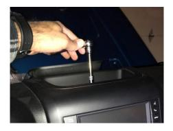
b. Remove the plastic kick panel below the steering wheel by pulling toward the driver seat and down from under the steering column. There are 4 tabs in the 4 corners & hinges at the bottom holding it on. Then Remove the two 7mm bolts located at the top on both sides of the steering wheel (circled)
