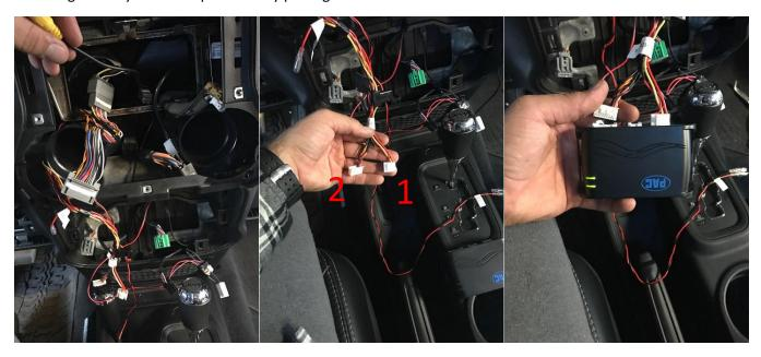
16. With everything working, tuck the BCI interface module into the open space next to the driver side vent (Blue circle) Then connect the black and red wires to the LED (they are clearly labeled. I taped them as well. I did not use the small red wire labeled "Camera power output". Then carefully tuck the camera power wires and LED wires down and out of the way then replace the HVAC panel. Be sure to reconnect all of the plugs!
