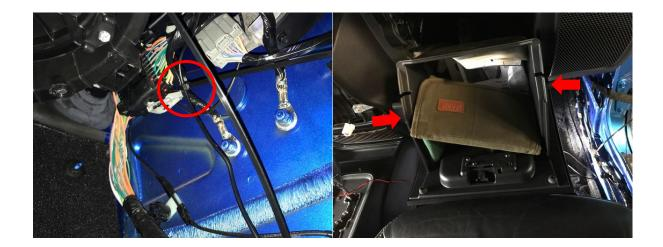
11. Bring the cable through the glove box toward the center counsel. There is a small passage you will be able to feed the yellow RCA & small black and red wires through. Route the Yellow RCA wire behind the plastic panels up to where the window switches are (3<sup>rd</sup> pic).
