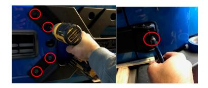
8. With the outside Hinge T-50 torx bolts tight, remove the 4 – 13mm bolts you replaced in step 7 and open the hinge & tighten the inside 4 – T-50 Torx hinge bolts.
