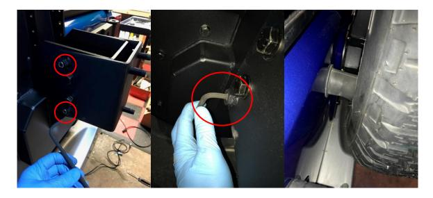
12. With your set screws tight, temporarily place the third brake light bracket in place on the carrier. Adjust the height according to the size of your spare. I was able to put some of the small 10mm bolts (without the locking nuts) in to keep it in place.
