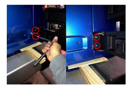
9. Now take your HD carrier out of the box and position it in place & thread in the 8 – 13mm Short carrier bolts (with washers) that came with it, starting with the 4 on the driver side. (1st pic). Use the 4 – 13mm hex bolts (with washers) that came with the hinge to secure the hinge to the tailgate. (2cnd pic). Locktite & Fully tighten all of these bolts! Tip: Get all of the bolts started by hand and tighten them evenly, small amounts at a time.
