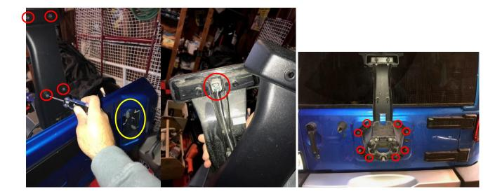
3. With your tailgate closed, remove the stock tire carrier by removing the 8 – 13mm bolts. (Circled above) Put to side. Remove the plastic hinge covers; up and towards the driver side for the tailgate covers & pry the top and bottom away from the hinge and push toward the passenger side for the hinge covers. Now place shims under the gate until they are tight. KEEP TAILGATE CLOSED FOR REMAINDER OF INSTALL.
