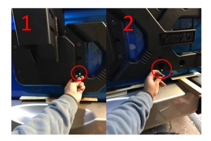
10. With the carrier and hinge completely tightened, you will now attach the lug plate to the carrier. Using a 19mm socket and 19mm wrench (or adjustable wrench) tighten the 4 – M12 bolts & Lock nuts almost entirely, allowing you to adjust the lug plate with some force.
