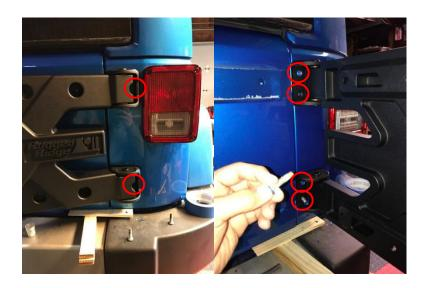
7. Now replace 4 – 13mm factory carrier bolts to help line up the carrier. Snug these in place but do not overtighten. With those snug, Tighten the outside T-50 torx hinge bolts.
