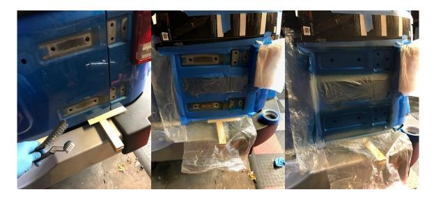
6. Time to mount your Rugged Ridge hinge. A second set of hands would make this easier. Hold the carrier in place and replace the factory T-50 torx hinge bolts; 2 outside, then open the hinge and replace the 4 inside. Apply Loctite to these bolts. Snug only, do not tighten down yet.
