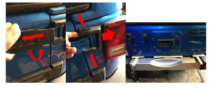
4. Next you will remove your factory hinges by removing the 4 - 13mm bolts on the tail gate. Flip the hinges to the open position and remove the T-50 torx bolts holding the hinges to the body/tub.
