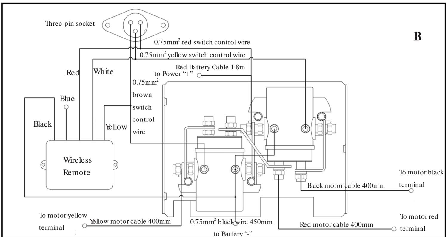
**SOLENOID BOX ASSEMBLY(12V/24V)PARTS LIST( If your winch is without wireless remote control, please ignore the remote and the relative wiring!)**
