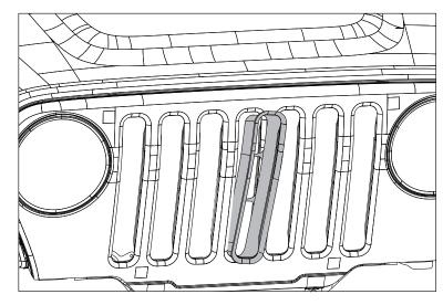
3. Press lower retainers into grille shell and press top of insert until clipped into place.
