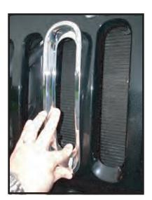
Clip lower retainers behind grille shell, and then push the top in until it clips in place. This usually can be accomplished by simply pushing on the insert, but sometimes it is helpful to squeeze the insert to the grille shell as shown.
