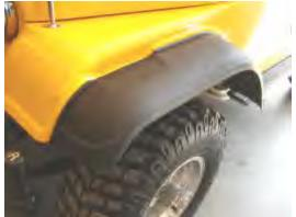
The new flare bolts in place easily and quickly utilizing the existing holes from the OE flare. This is the left front. Simply repeat the process on the right side and you're halfway finished.
