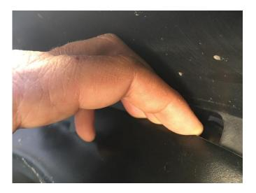
4. Once I had each hole lined up I used the provided push rivets and inserted them into the holes to secure the fender to the Jeep.
