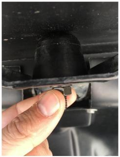
2. Next I carefully popped off the push rivets that were previously installed on the fender liners. This was easy, but took just a little time. I used a flathead screwdriver to do this. Once the push rivets on the top of the liners were removed I simply pulled the liner away from the body and inserted the fender flare between the liner and the body of the Jeep.
