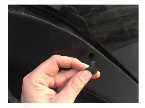
3. Once I had the fenders inserted between the body and the fender liner, all I had to do was line up all the holes, which only took a little work. Most holes lined up without any issue, some I used a flathead screwdriver to just line the holes up.
