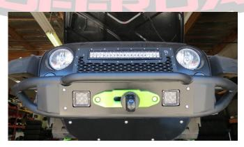
6. Check, and re-tighten if needed, all mounting bolts after 100 miles and periodically thereafter.
