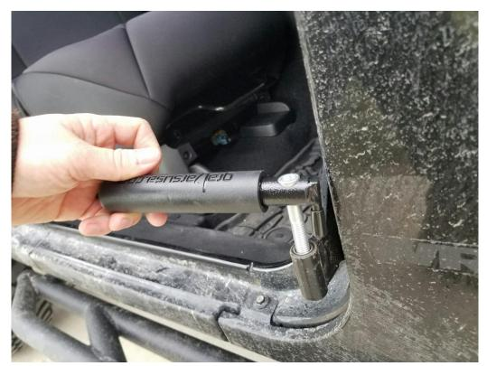
7. Put a supplied washer and nut on the bolt. Tighten with 5/16" Allen wrench and a 9/16" socket. You don't need it super tight, just enough to keep it from rattling around.
