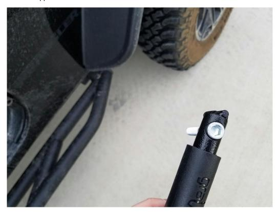
6. Insert the bolt into the lower door hinge as shown. If you have the correct Bar for this side the rubber nub will be offset toward the front of the Jeep.
