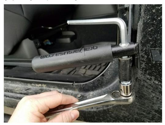
8. Rotate the BootBar fully forward and it's ready to go! Complete Steps 1-8 on the other side.
