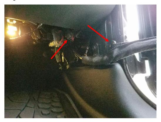
4. Open the door and remove it. You can hold onto the outer door handle and the bottom of the door. It is also helpful to have the window open so you can hold onto the top. Make sure you have a place to put the door that will protect it before you remove it, it is heavy and difficult to maneuver.
