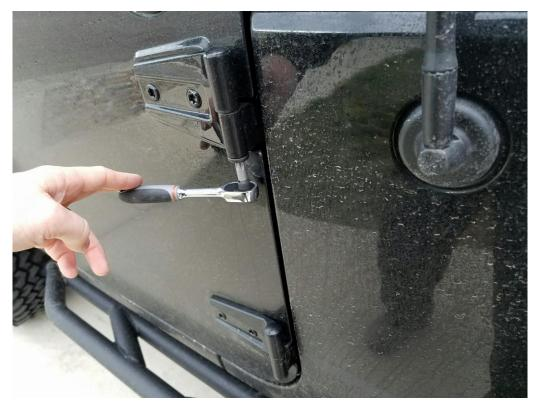
2. Make sure to fold your mirror in prior to disconnecting the inside door connections or the door could swing and dent the outside. Opening the window can also help with removal in a later step
