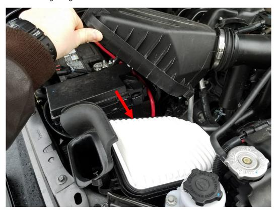
**4.** Then insert your new AEM Dry Filter as shown below. The bulk of the filter should be facing downward. Make sure the rubber seal is fully seated around the edge.
