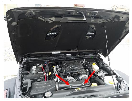
2. Using your hands, unclip the 4 metal clips holding your air box closed.
