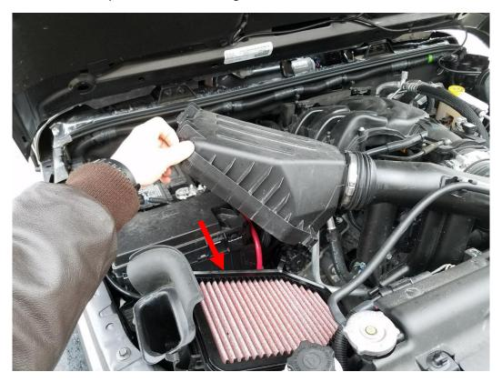
5. Place the top back on the air box, making sure it gets a good seal all the way around. It helps to start by seating the right side first then work your way toward the air inlet. Now connect the 4 metal clips around the air box. Be careful not to break the clips off. If it is difficult to clip them, the air box might not be fully sealed.
