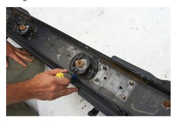
Step 4: Wire LED Pigtail. Blue wire to factory black wire. Brown Wire to the factory White or white and red wire.
