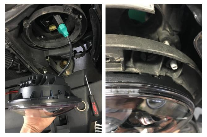
7. Place the bezel back around the headlight and use the torx #15 screwdriver to tighten the 4 screws back into place on each headlight.
