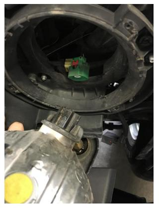
5. Assemble the wiring harness with the anti-flicker module that is included with the headlights as shown below. Plug directly into the factory wiring harness that is still in the jeep and then push the red clip down to relock the harness into place (If the red clip gives any trouble, this is where pliers were used to gain more leverage).
