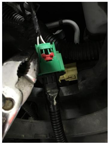
6. Take the other end of the harness and now plug it into the new Raxiom led headlight. Place the headlight into position and realign the plastic tabs so that the headlight sits flush in place.
