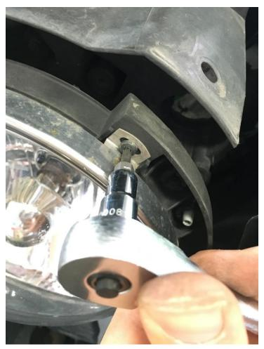
4. Remove factory headlights by unplugging each from the wiring harness and set them aside.
